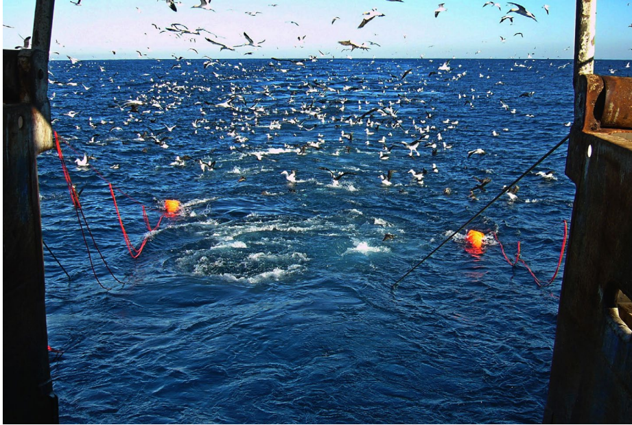
Figure 7.A Bird-scaring lines (in orange) keep a variety of albatross, petrels, and gannets at a safe distance from the baited hooks deployed off a trawler off South Africa. Photograph by BirdLife South Africa Albatross Task Force Programme, CC BY 4.0.
