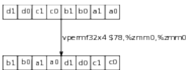
Figure 7.6 Effect of applying the vpermf32x4 instruction to a ZMM register. Each entry shown is a double-precision number.
