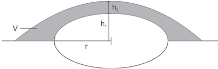
Figure 3. Visual explanation of the variables used in the formula to calculate the volume ( $V$ ) of material pushed up by the ice lens. When the pingo disintegrates and becomes a pingo scar, the volume of material will make up the rampart.
