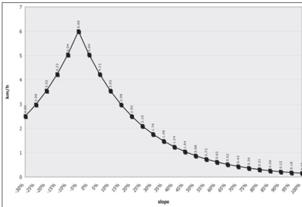
Figure 3. Graph of the walking speed (km/h) based on slope, calculated with the Gorenflo/Gale algorithm.
