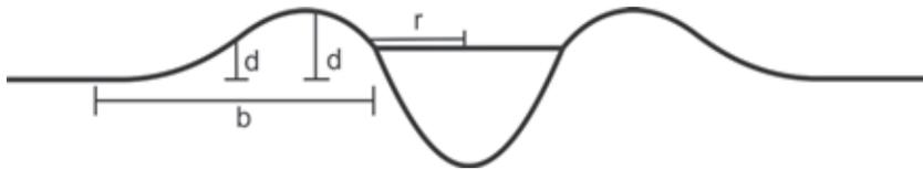
Figure 2. Visual explanation of the variables used in the formula for calculating the scope of a rampart.
