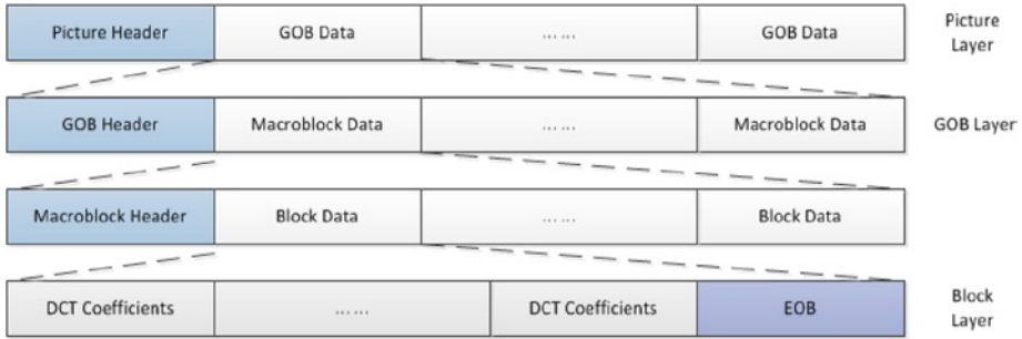
Figure 3-2. Data structures of the H.261 video multiplex coder
