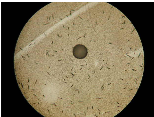
Figure 3. Track-etch prints of a U-oxide particle, ( ^{235}\text{U}/^{238}\text{U} 0,25), NIST sample 3, 500 \times magnification.
