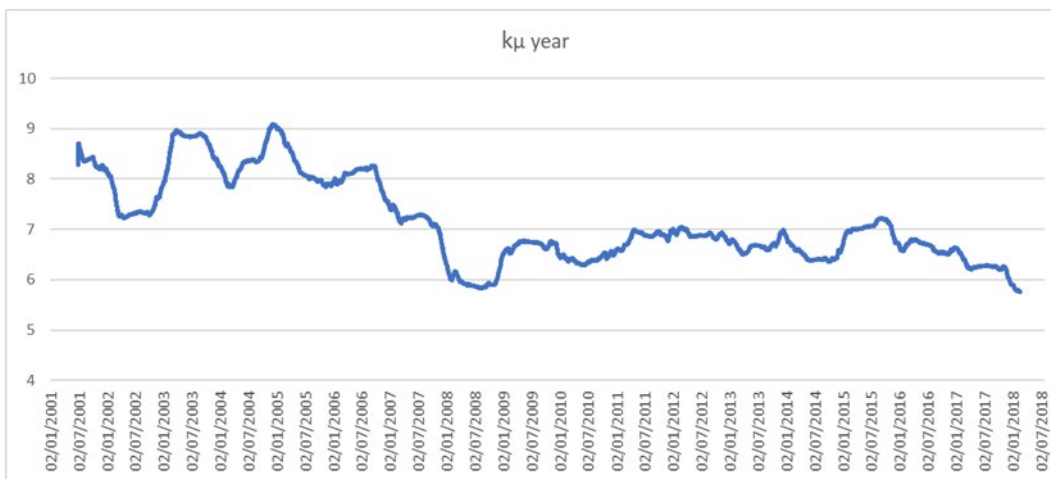
Figure 6. Parameter k_{\mu_{year}} for the flowmeter QX00111 between 2001 and 2018
