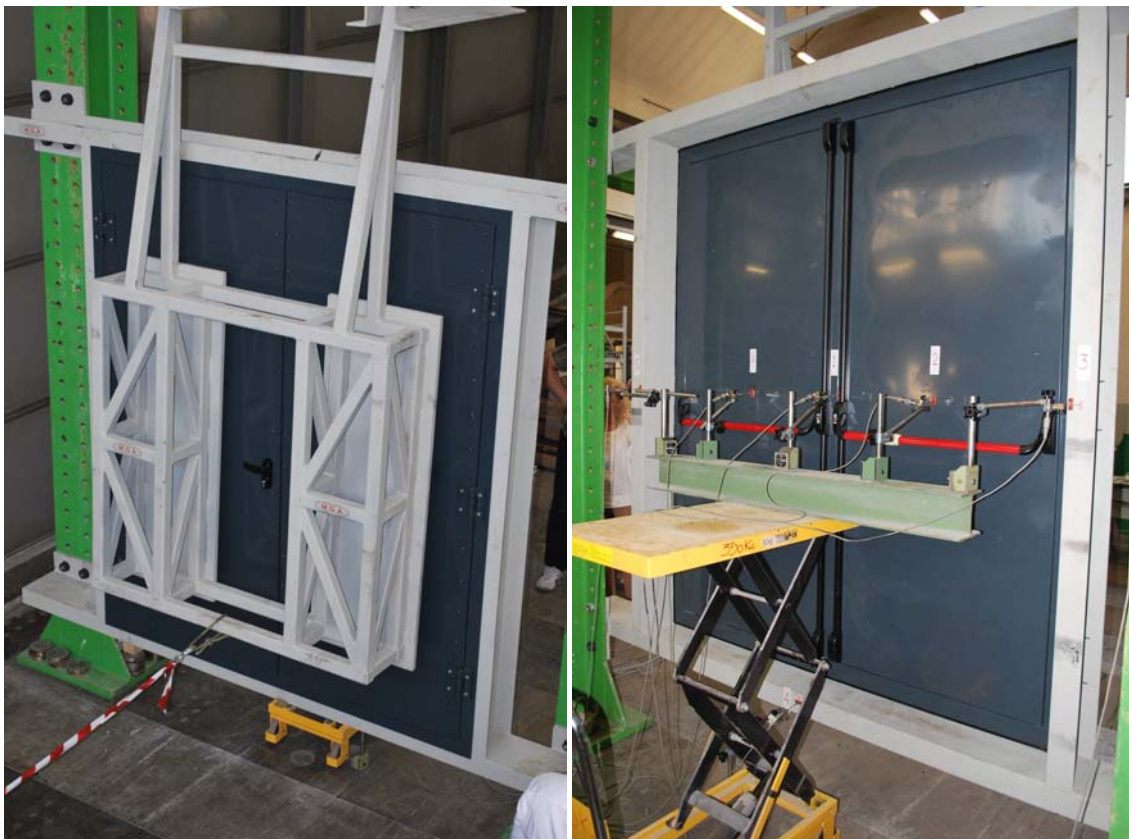
Figure 12: Test set-up: impacting element (left) and position of displacement transducers (right).
