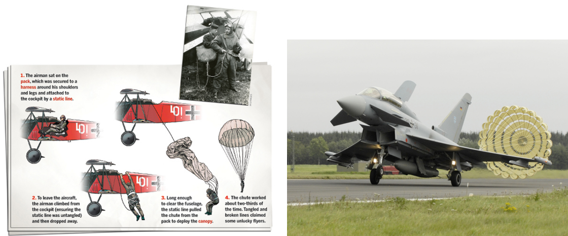
Figure 1.2: Heinecke escape (left) [7] and Eurofighter Typhoon ribbon (right) [8] parachutes.
