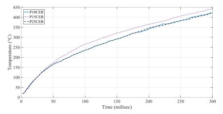
Fig. 7 Behavior of temperature in the zone of the cutting edge radius
