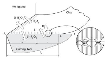
**Fig. 3** Contact configuration and heat sources in the tool-chip-workpiece system, adapted from [10]
