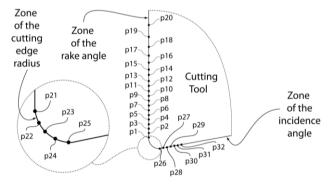
Fig. 5 Discretization of the cutting tool by zones
