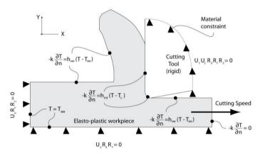
Fig. 4 Modeling of orthogonal cutting with coupled Eulerian-Lagrangian method
