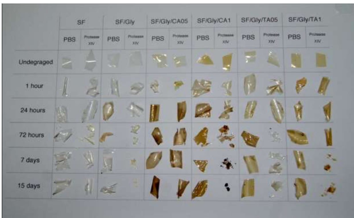
Figure 3.5.1 – Macroscopic evaluation of the samples before and after incubation in either PBS, or protease XIV (derived from Streptomyces griseus , 0.693 U.mL -1 ), up to 15 days.
