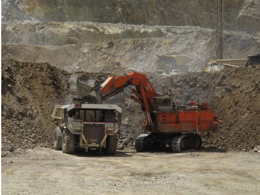
Pala frontal - Hydraulic front shovel
