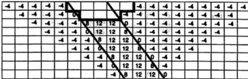
Figure 5.70. Situation after floating down two rows.
