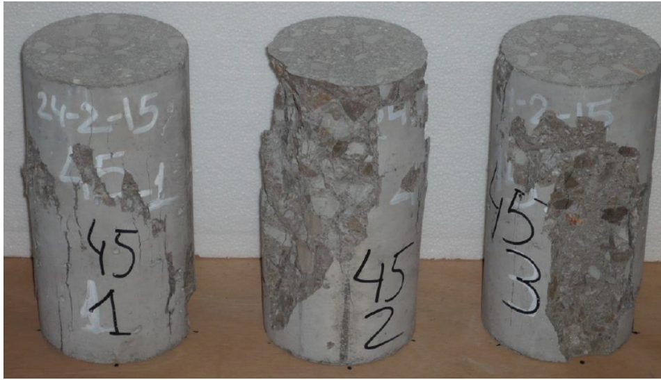
Figure 4: Specimens after the UCS test
