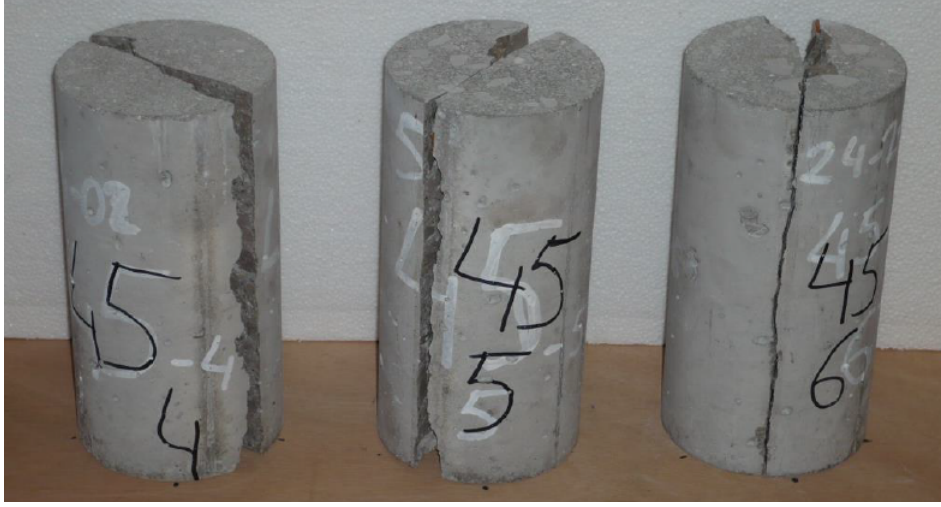
Figure 6: Specimens after the BTS test
