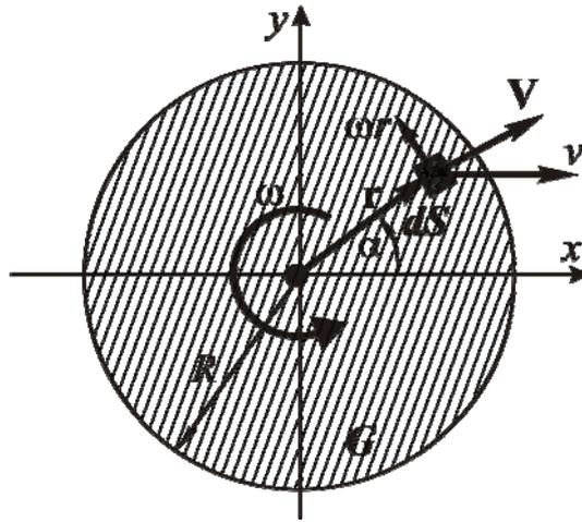
**Figure 1.** Kinematics inside the contact spot letters
