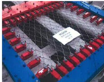
Figure 2: A TECCO type net is pulled in mesh direction decreasing the mesh angle while deforming.
