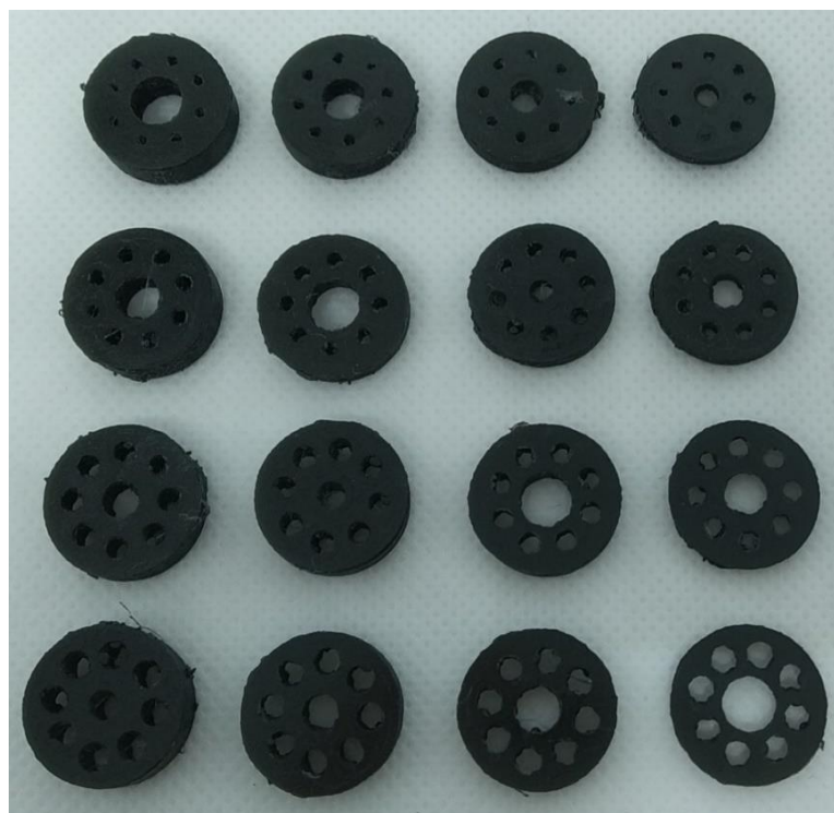
Figure 15. Detailed picture of drilled plates manufactured by 3d printing AM method. Flowrate was measured using NATRAIN partial counter. This device registers total litres as absolute variable. The author used an interval of 25 seconds in order to calculate the flowrate through the system. Final model is presented on figure 16.
