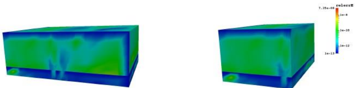
Fig. 4: Relative error of the expectation of the electrical field in a coplanar waveguide after using a pMOR Krylov-space technique within Uncertainty Quantification based on generalized Polynomial Chaos expansions.
