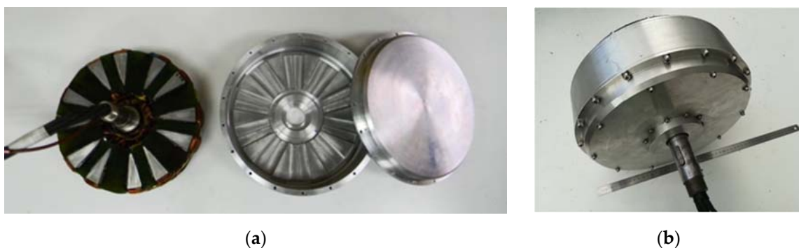
Figure 16. (a) Stator and the two motor covers, showing in the central part the SMC rotor pieces glued on the cover and (b) view of the fully assembled AFSRM prototype.
