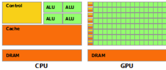
Fig. 1. Comparison of CPU and GPU hardware. GPU includes more ALUs for data processing (from [10]).
