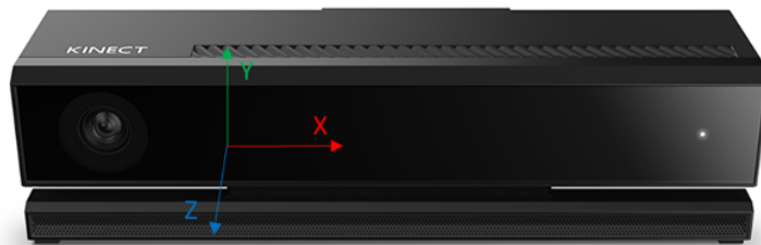
Figure 3.2: Coordinate system of the Kinect devices. [18]
