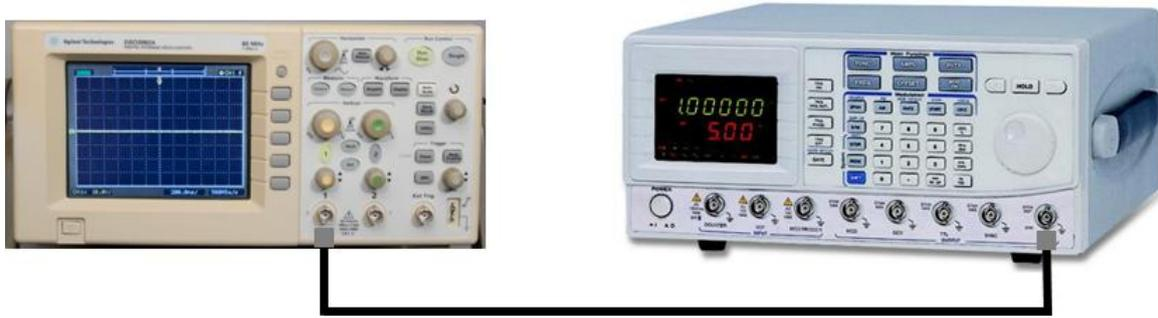
**Figure 18.** Oscilloscope connection for visualizing time-varying signals from the waveform generator.
