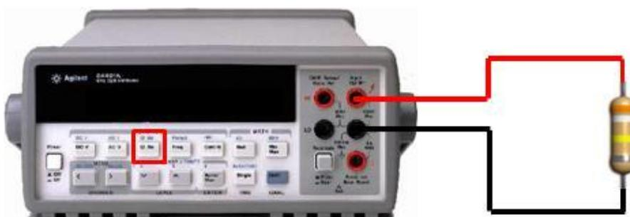
*Figure 3.* Output connection and multi-meter configuration for measurement of electric resistance.
