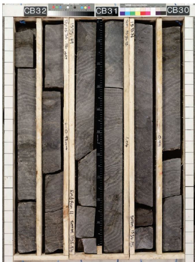
Fig. 3. Example photograph of slabbed core, showing contorted bedding of banded polyhalite with magnesite and anhydrite, ~1,535 m, borehole SM3A. Scale at the side of the core is in 5-cm intervals.
