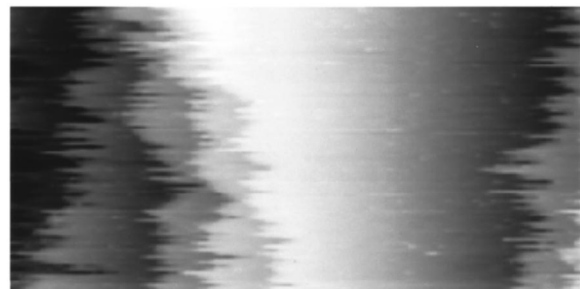
FIG. 1. STM image of the clean Ag(110) surface at 300 K with fluctuating steps ( 340 \times 180 \text{ \AA}^2 , V = -0.5 \text{ V} , I = 0.1 \text{ nA} ).
