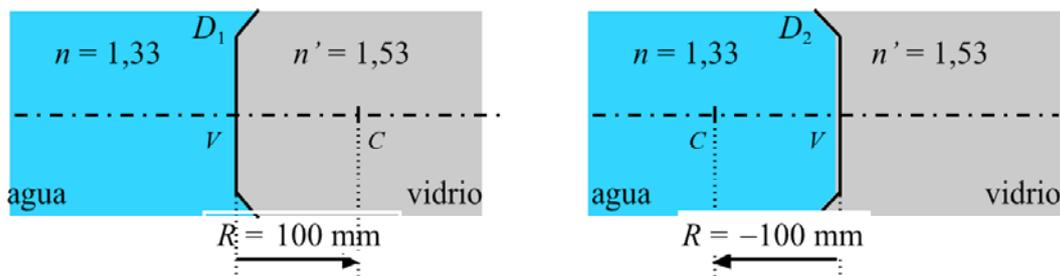
R/  $D_1$ : Lente delgada con:  $P'_1 = 2,00$  D ;  $\overline{f'_1} = 500$  mm;  $\overline{f_1} = -500$  mm.
