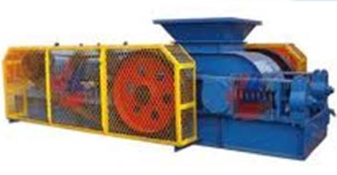
Fig. 6.1. Schematic Diagram of Roll Crusher
