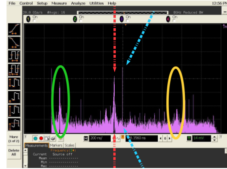
FIG. 8. FFT of the signal corresponding to the fabricated circuit. Proof of the one sideband cancellation at 3.6 GHz.
