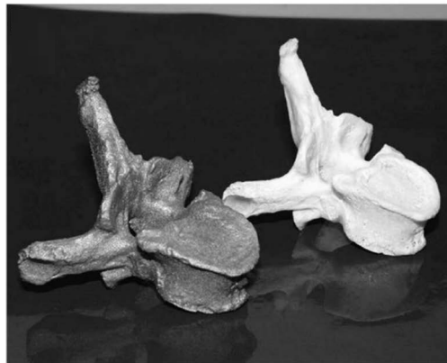
Figure 7. Printed spinal titanium alloy prosthesis obtained with the SLM technique [154]. Reprinted from Biomaterials , 27, Dirk A. Hollander, M.von Walter, T.Wirtz, R.Sellei, B.Schmidt-Rohlfing, O.Paar, H.-J.Erli, Structural, mechanical and in vitro characterization of individually structured Ti-6Al-4V produced by direct laser forming, 955–963, Copyright (2006), with permission from Elsevier.
