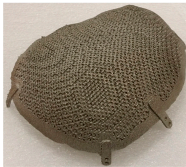
Figure 5. Cranial implant 3Dprinted in titanium with the EBM technique [140]. Reprinted from Electronic Journal of Biotechnology, 29, K. Moiduddin, S. Darwish, A. Al-Ahmari, Sh. ElWatidy, A. Mohammad, W. Ameen, Structural and mechanical characterization of custom design cranial implant created using additive manufacturing, 22–31, Copyright (2017), with permission from Elsevier.
