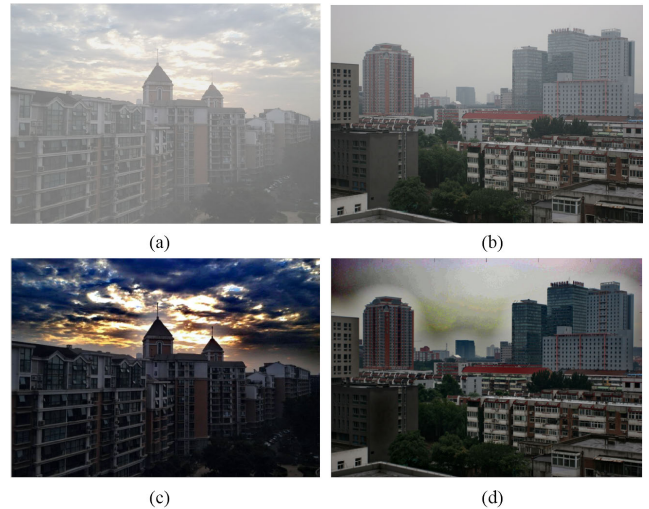
FIGURE 1. Examples of the main drawbacks of DCP method. (a) Input image 1, (b) input image 2, (c) restored image from (a) presenting saturated sky regions, (d) restored image from (b) illustrating image artifacts.
