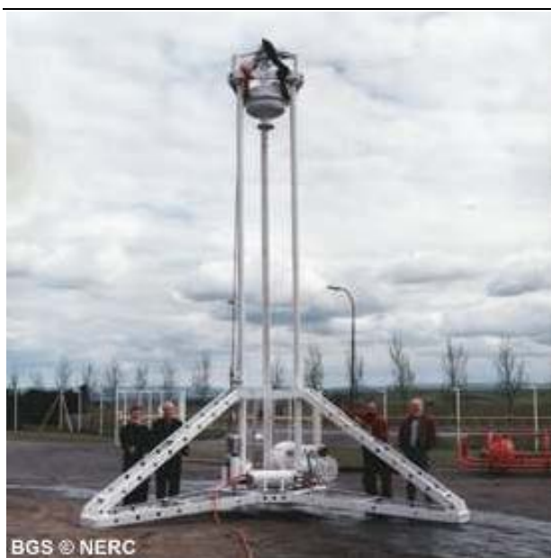
Fig. 2. The British Geological Survey 5m Rockdrill (RD1) first developed in 1982 and is still used to recover cores today.
