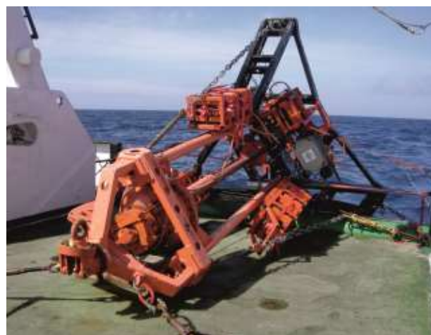
Fig. 3. The British Geological Survey 3m configuration of the battery operated vibrocorer on its side on-board the R/V Belgica .
