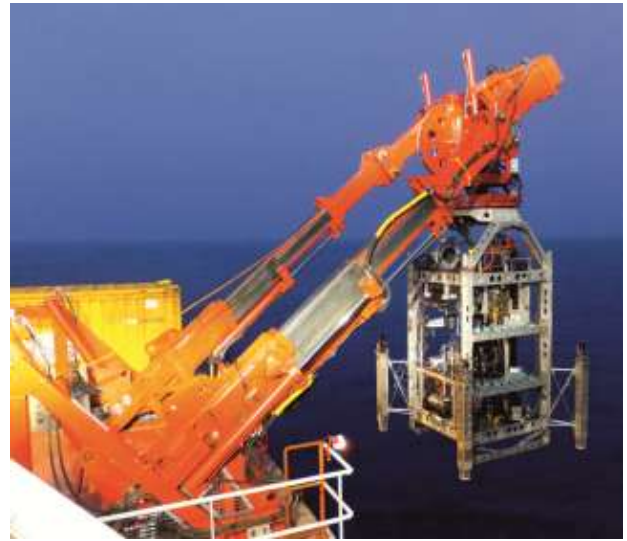
Fig. 4. The British Geological Survey 55m remotely operated seabed rock drill (RockDrill2) being deployed in the Sea of Japan.
