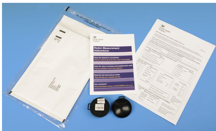
Figure 9. PHE standard pack of passive radon detectors
