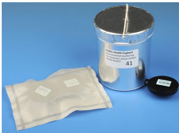
Figure 10. PHE outdoor radon monitoring pack
