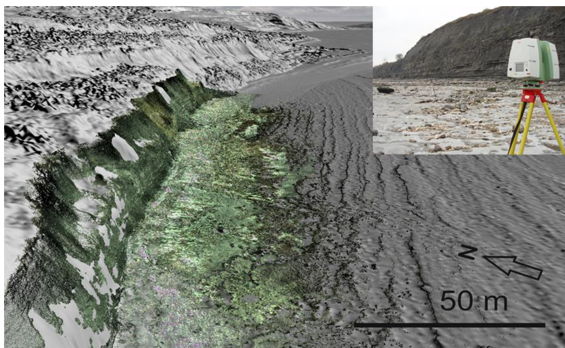
Figure 2. Features of coastal landslides in Monmouth Ledges, Lyme Regis, West Dorset. Inset: Laserscanner mounted on tripod.
