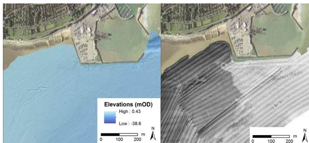
Figure 3. Seabed substrate differentiation and detection from [a] bathymetry and [b] backscatter datasets (Ramsgate, Kent, UK).
