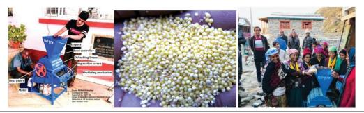
Figure 2. Electric proso millet dehusker testing at Khumaltar and field testing in Humla.
