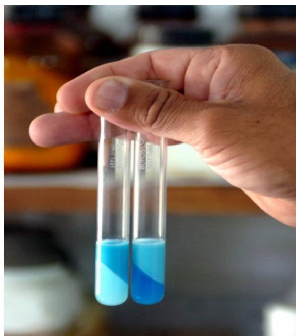
Fig. : Comparison of developed color in presence and absence of detergent in milk. Relatively more blue color in lower layer (right side tube) than upper layer indicates presence of detergent in milk.
