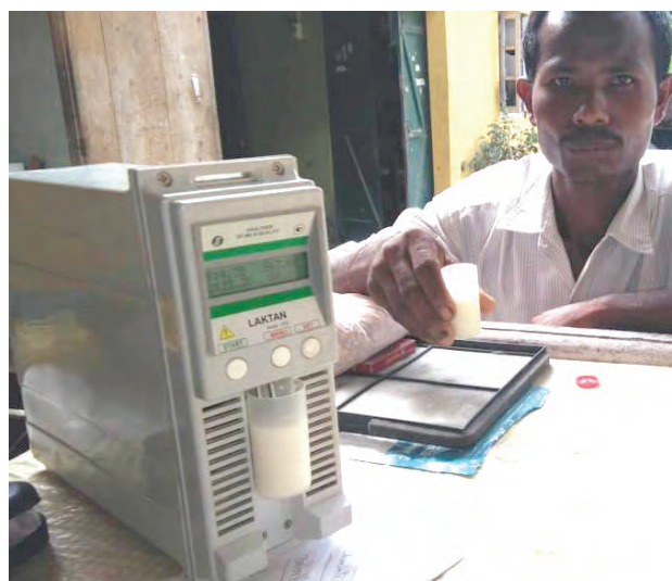
Milk is being tested by using a digital Milk Analyzer
