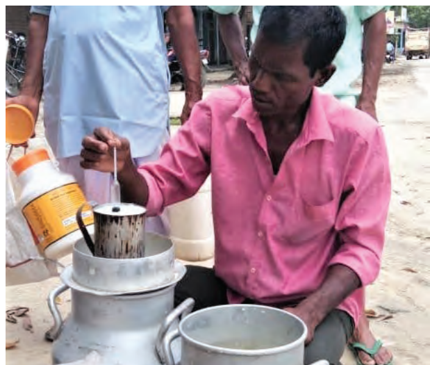
Milk is being tested by using manual lactometer
