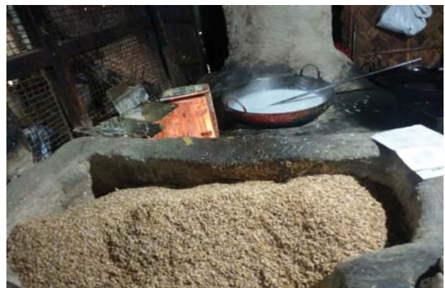
Rice bran commonly used as fuel in the cottage product making unit in Assam
