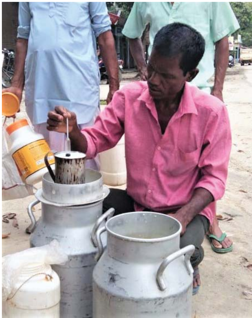
Milk is being tested by using manual lactometer
