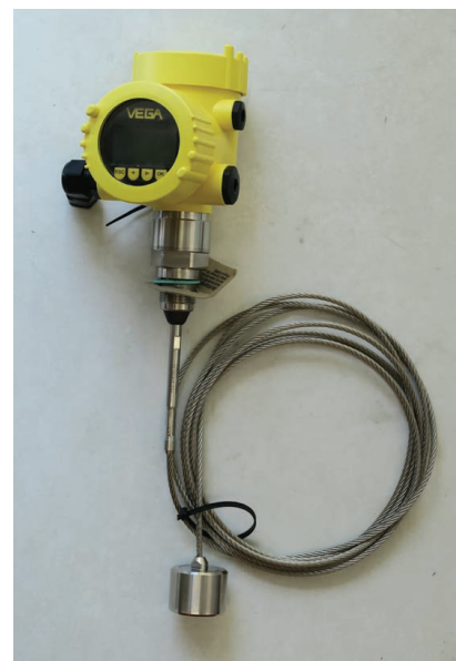
Figure 4 The radar gauge for installation at Rothera. This unit emits high-frequency microwave pulses which are reflected by the sea-surface, allowing the height above sea level to be inferred from the transit time between emission and detection of the signal. The pulses are guided down the stainless steel cable to prevent them from reflecting off the walls of the stilling well and the cable itself is weighted to minimise vertical movement.
