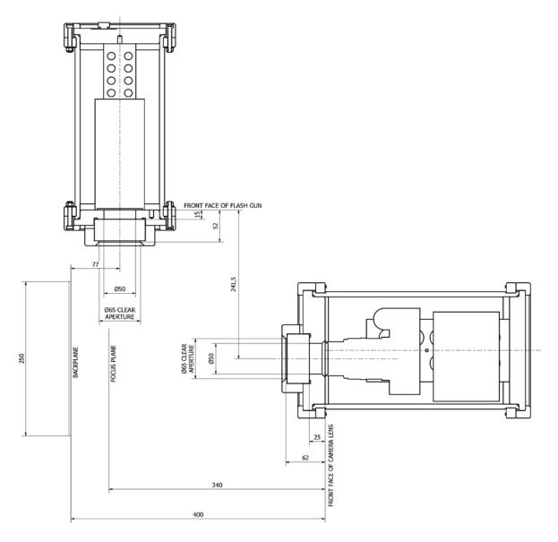
Figure 22 Camera and flash geometry layout (plan view):
