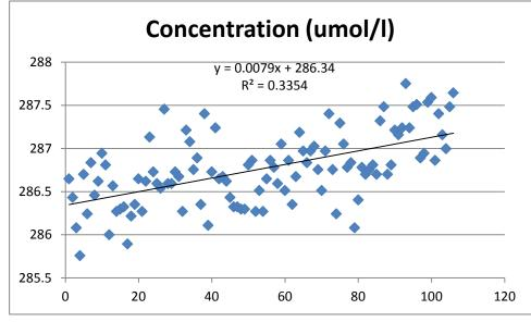
*Figure 7 Example of measurement from Setup I. Uncorrected start concentration from CTD 11 at 5m depth.*
