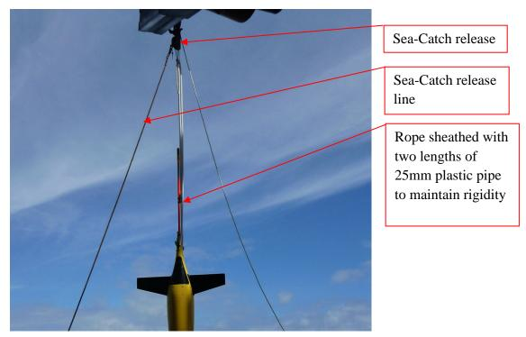
Figure 57 Deployment using Rigid Rope and Rexroth winch
