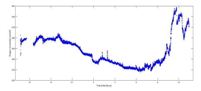
*Figure 8 Uncorrected oxygen concentration measured form setup II over the course of 24 hours. The gap around 15:00 is due to electrode problems.*
