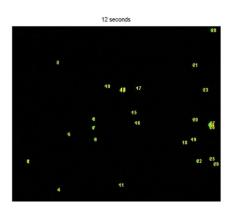
Figure 12 Example of three images obtained during deployment 1 of PELAGRA P4 at ~01:00h. The images are at 8, 10, 12 seconds after ~01:00h and shows a range of particles sizes sinking with a vertically downward movement through the illuminated slab of water. The particles are sinking freely in the water column, undisturbed by the presence of the PELAGRA. Only the use of a neutrally buoyant platform can provide recordings of freely sinking particles.
