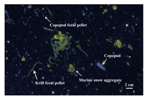
Figure 9 Small section from a gel trap deployed at 100 m depth during the DF-6 deployment. The shape and structure of all particles collected in the gel is preserved and can be used to identify particle types and measure their sizes.
