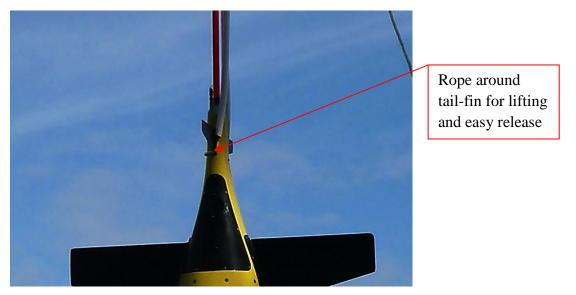
Figure 58 Close up of deployment sling showing attachment around tail-fin for ease of release
