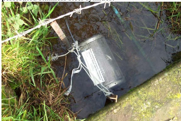
Figure 4. POCIS deployed in a stream (Farm 8 downstream) inside its perforated stainless steel cylinder.
