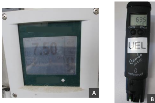
Figure 27 – Equipment used to measure pH. A – Equipment linked to a probe and a signal converter that measures pH and temperature; B – Portable pH meter.
