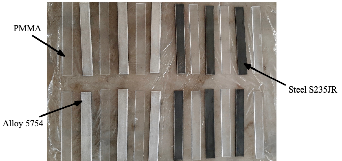
Figure 3.5: Different material samples used (before bonding).
