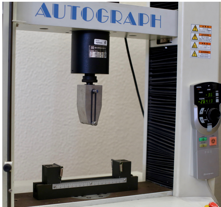
(a) 3PB device coupled to the testing machine.
