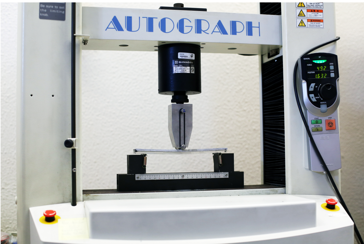
Figure 3.11: Laminated beam under a 3BP test.
