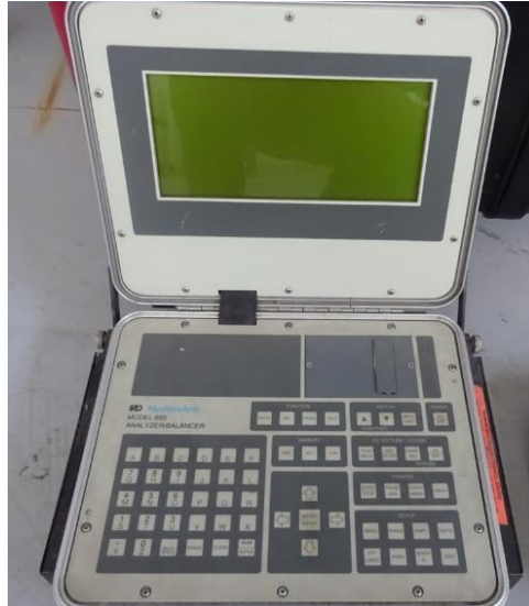
Figure 19- IRD Mechanalysis - Model 885 – Analyzer / Balancer
