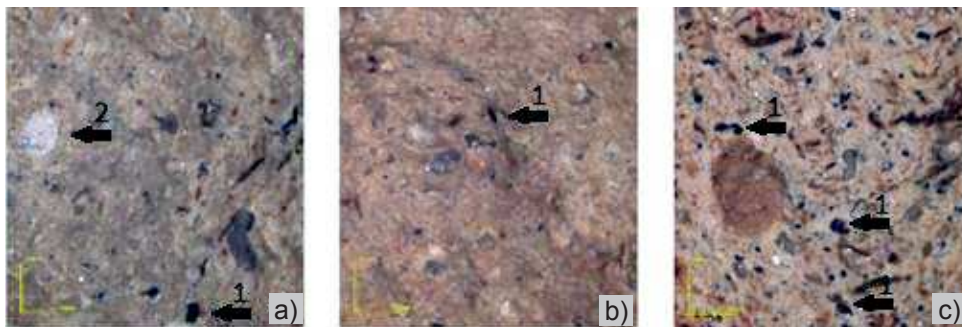
Figure 8. Confocal optical microscopy of the ceramic masses with 15% ORW incorporation in strong clay (AF15) sintered at 850 °C (a), 950 °C (b) e 1,050 °C(c).
