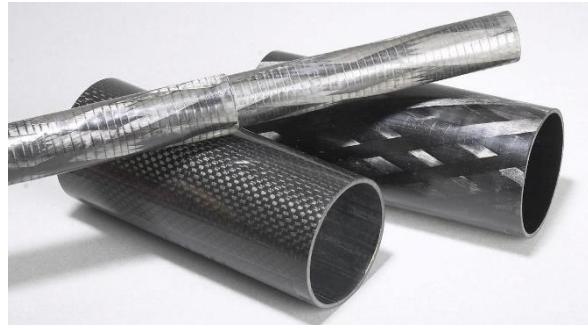
Figure 58: Typical products from the classical filament winding technique
