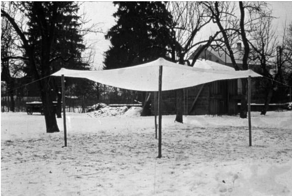
Figure 7: The hanging membrane model shown in Isler's IASS Congress paper, 1959
