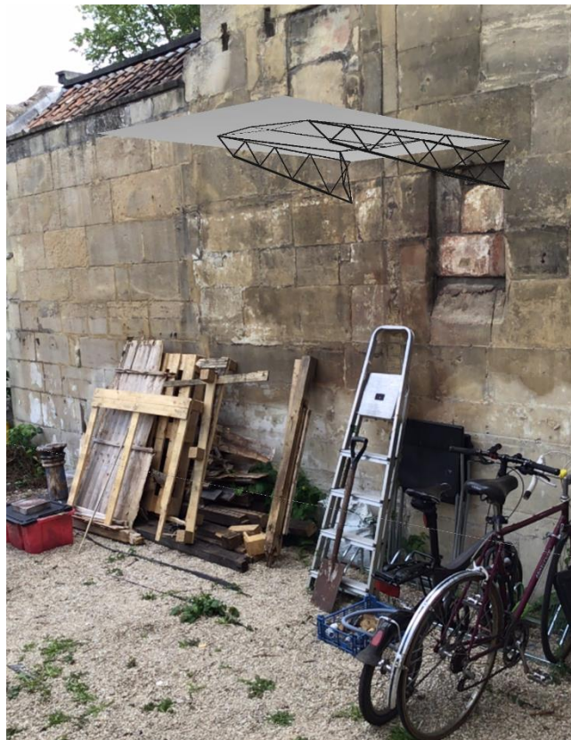
Figure 72: Using augmented reality to see the final geometry for one module of the canopy
