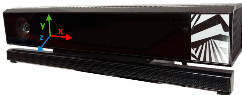
Figure 2. 3-D coordinate system of the Kinect v2, located at the center of the infrared sensor [26].
