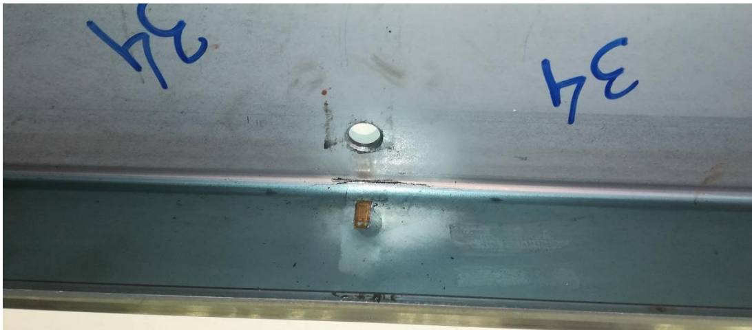
Figure 80 - Representative fatigue cracks (specimen 34 example).
