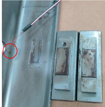
Figure 53 - Load actuators for downward loading scenario setup #3 (strain gauge marked in red).
