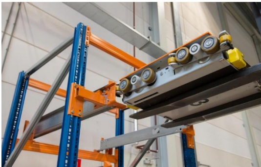
Figure 21 - A shuttle being placed onto its tracks, Z-rails (courtesy of NEDCON).
