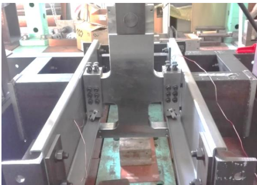
Figure 30 - Experimental fatigue testing setup for Z-rails (laboratory).
