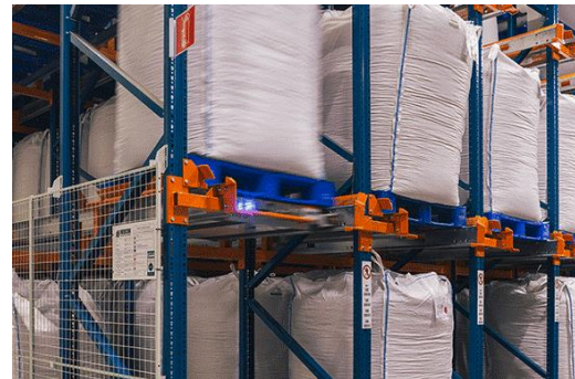
Figure 22 - A loaded shuttle moving along Z-rails (courtesy of NEDCON).
