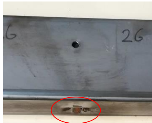
Figure 67 - Strain gauge's placement for upward loading scenario setup #1.
