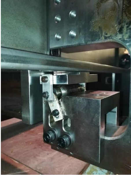
Figure 78 - Load actuators for upward loading scenario setup #3.
