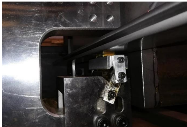
Figure 72 - Load actuators for upward loading scenario setup #2.
