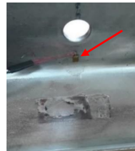
Figure 39 - Strain gauge's placement (downward setup #3; in setup #1 the shown drilled hole is not present).
