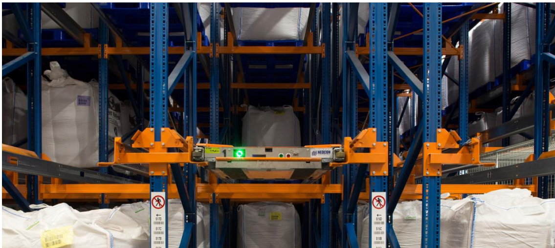
Figure 20 - Z-rails in a rack structure prepared for shuttles (courtesy of NEDCON).
