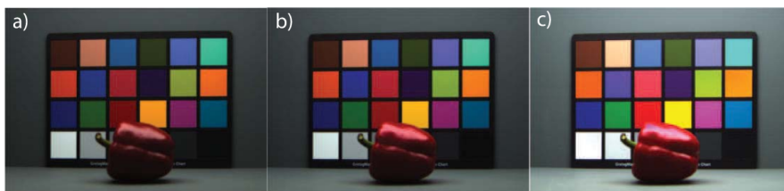
Figure 2.1: a) Photo captured with sRGB sensors, b) Photo captured without sRGB sensors, but color corrected to sRGB using polynomial model, c) Same color correction applied after intensity of light increase [9].
