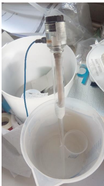
Figure 7 – Illustration of the set-up used for the RE in the UPD tests.
