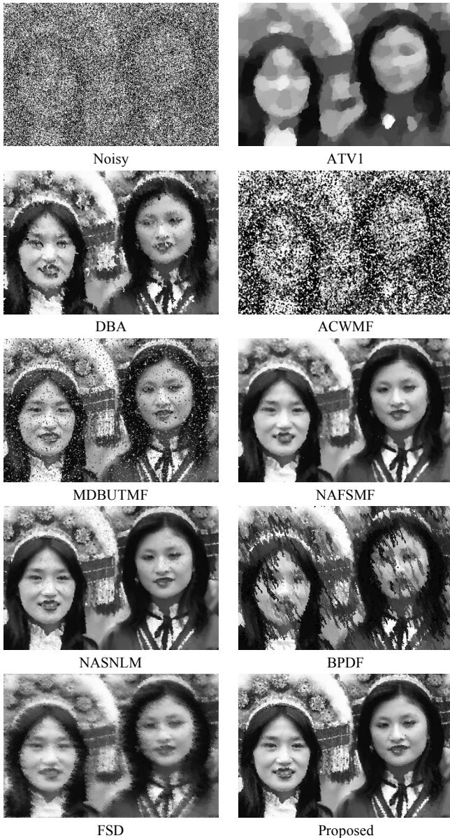
Fig. 4. Denoising results for image “189003” with noise level of 80%. The PSNR/SSIM value of the noisy image is 5.57764/0.018569; the denoised images by ATV1 is 16.403/0.50677, DBA is 17.56/0.58897, ACWMF is 7.19594/0.049072, MDBUTMF is 16.5782/0.3789, NAFSMF is 21.1193/0.72084, NASNLM is 21.6852/0.72489, BPDF is 13.8834/0.41728, FSD is 16.978/0.50546 and the proposed method is 21.9649/0.7818.
