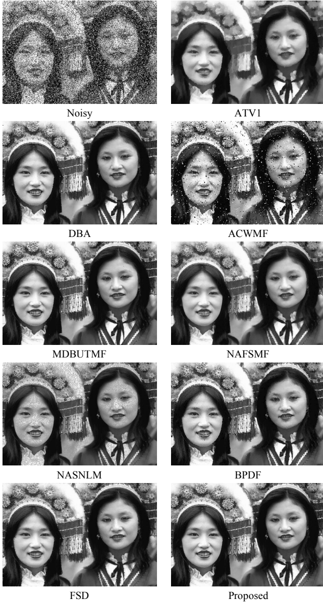
Fig. 2. Denoising results for image “189003” with noise level of 40%. The PSNR/SSIM value of the noisy image is 8.5836/0.084868; the denoised images by ATV1 is 22.7285/0.77244, DBA is 25.6268/0.90624, ACWMF is 17.2833/0.52407, MDBUTMF is 27.3143/0.93063, NAFSMF is 25.167/0.89268, NASNLM is 20.7238/0.75841, BPDF is 24.2967/0.87242, FSD is 25.4715/0.89481 and the proposed method is 27.3823/0.93455.
