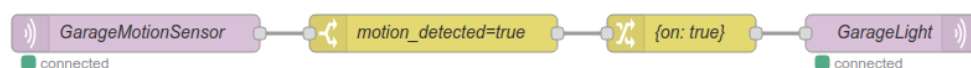
Figure 6.4: Resulting flow for scenario “When there is movement in the garage, turn on the garage lights”
