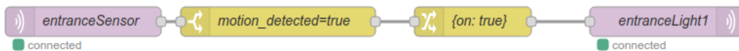
Figure 5.2: Node-RED flow for “when there is motion in the entrance, turn on entranceLight1” variation
