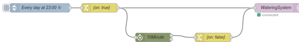
Figure 6.8: Resulting flow for scenario “When it is 23:00, turn on the garden watering system for 10 minutes”
