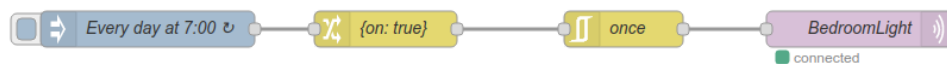
Figure 6.9: Resulting flow for scenario “When it is 7:00 today, turn on the bedroom lights”
