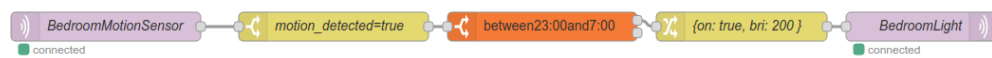
Figure 6.6: Resulting flow for scenario “During night, when there is motion in one room, light that room at 200 brightness”
