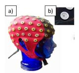
Figure 2. 3: a) EEG head cap with electrodes "already-assembled"; b) Gel-based electrode. Adapted from [129].
