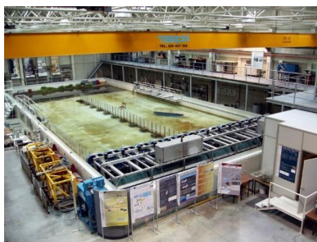
Figure 23 - Wave tank installed in the Hydraulic Laboratory at FEUP [33]
